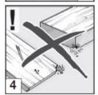
The subsurface on which the panels are to be installed must enable the floor panels to be installed in accordance with the manufacturer's instructions (product insert). Mineral subsurfaces (e.g. screed, water-based heated screed, concrete, asphalt) count among the suitable subsurfaces. Please note that substructures must comply with the generally recognised rules for dry constructions in wet rooms.
